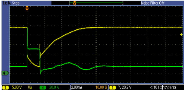
Short @ Vin = 24 VDC, Load = 800 W, 1 st IC303_1
