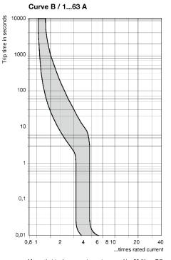
Magnetic tripping currents are increased by 30 % on DC supplies. Ambient temperature 30  $^\circ\mathrm{C}$
