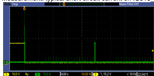
CH1 yellow: Output voltage 5 V/Div, CH4 green: Output current 10 A/Div, Timebase: 4 s/Div
